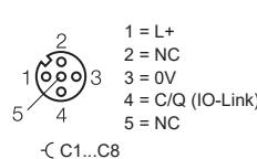
Power Supply Connector L-coded
