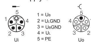
Note: U<sub>B</sub> is the module power supply, and U<sub>L</sub> is the load power supply
