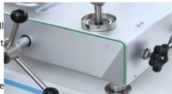
regulator needs to be slowly rotated to pressurize to prevent pressure overload;
